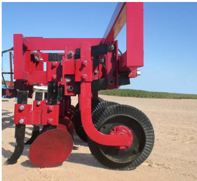
Fig. 2) Individual unit parallel linked showing coulter/gauge wheel and peel-off disks and mulching knife
